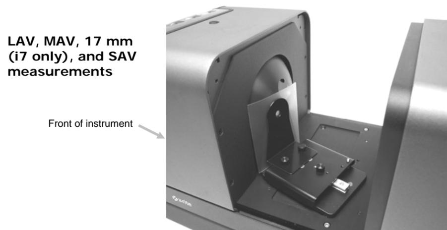
**Transmission holder at the lens (direct measurement) example**
