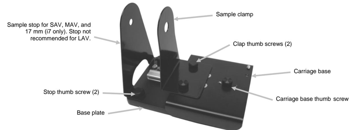
**Base Plate with Stop and Clamp Attached**
