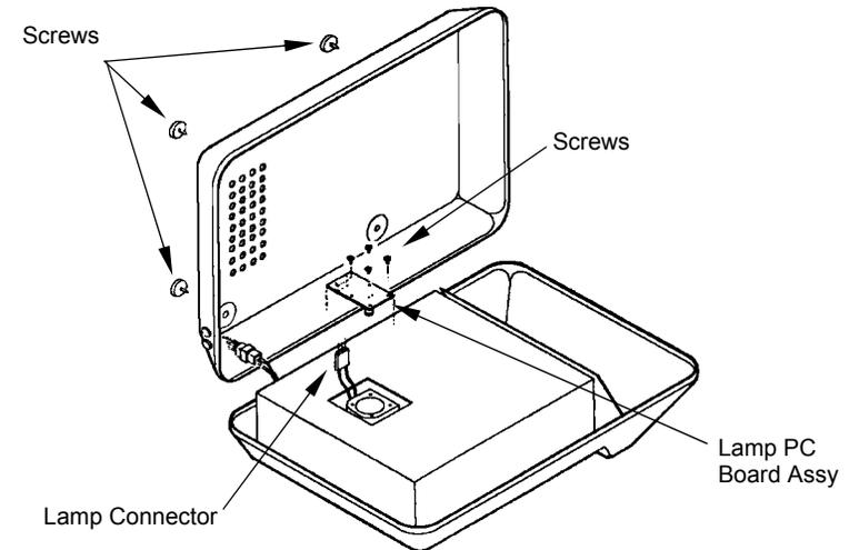
Figure 7. Lamp PC Board Access
