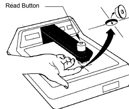
Figure 2. Aperture Removal
