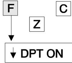
10. Press **[FUNCTION]** to advance to FUNCTION COMP. Each depression of **[ZERO]** key will alternate between COMP OFF and COMP ON.
