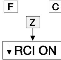
5. Press **[FUNCTION]** to advance to FUNCTION RPT. Each depression of the **[ZERO]** key will alternate between RPT ON and RPT OFF.
