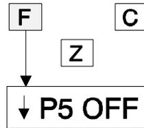
7. Press **[FUNCTION]** to advance to BAUD. Each depression of **[ZERO]** will page thru BAUD 2400, 4800, 9600, OFF, 300, 600, and 1200.
