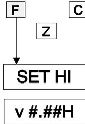
5. Enter the correct Cal Hi value for Visual (as marked on the step tablet) by pressing and holding  $\downarrow\uparrow$ (Zero) down and using the  $\downarrow$  (Function) key to decrease value or the  $\uparrow$  (Color) key to increase value. Then release both keys.
