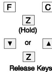
6. Depress **[COLOR]** key to select Ultraviolet cal value. Cal Hi value is displayed for Ultraviolet. (If value is correct skip to Step 8.)
