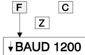
8. Press **[FUNCTION]** to advance to FUNCTION HDR. Each depression of **[ZERO]** key will alternate between HDR ON and HDR OFF.
