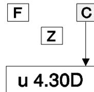
3. Measure the density to be zeroed, and keep the **[READ]** button depressed (thru Step 4).
