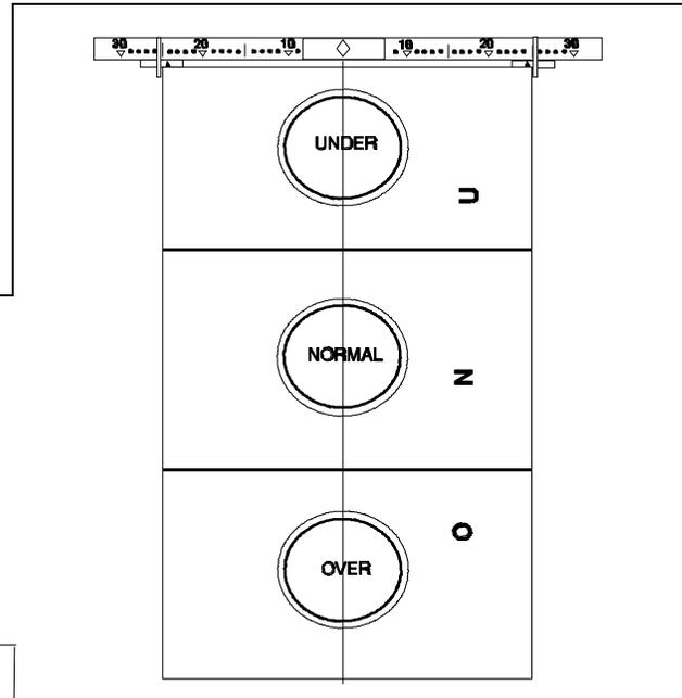
Step 4 - With "Under" end of strip facing unit, position strip with center of bull's-eye over middle diamond. Slide paper guides next to strip. Insert strip until it rests against the drive rollers.
