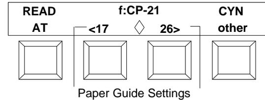
Step 4 - Align the strip with right guide (indicated by flashing right guide no.#) so you can measure the Cyan and Stain fields.
