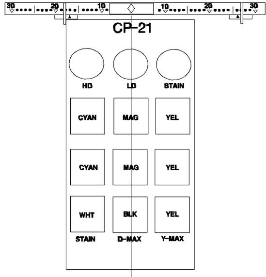
Step 6 - After 2nd pass complete, rotate strip and align it with the right guide so you can measure the Yellow field.
