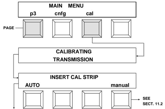
Step 2 - Insert the Auto-Cal strip into the 35mm slot until it rests against the drive rollers. The strip indicates which end to insert.
