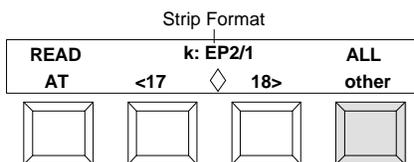
Step 3 - Adjust the paper guides according to the numbers displayed.
