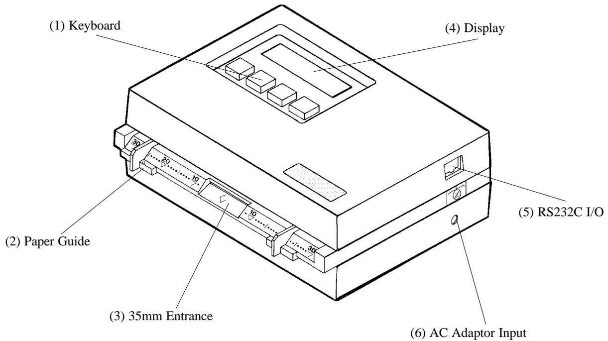
(1) **KEYBOARD** - Consists of four keys and is used for selecting control strip format (paper, film, & printer balance), viewing/transmitting data, and various mode functions.
