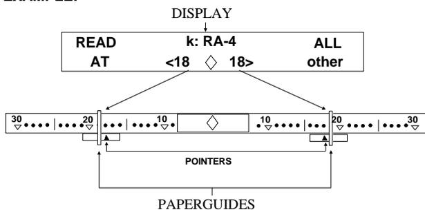
To move the paper guides to the desired location, lift-up on bottom slightly and slide left or right (see below).
