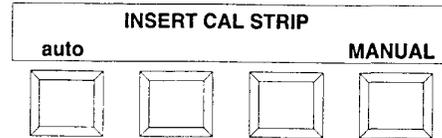
Step 6 - Insert the Auto-Cal strip into the 35mm slot until it rests against the drive rollers. The strip indicates which end to insert.
