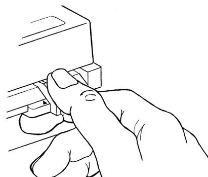
To accommodate 35mm wide strips, the 880 has a special stationary guide located above the diamond.
