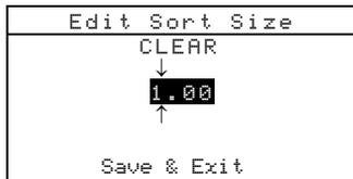
4. Use the Tab keys  $\updownarrow$  to choose the desired digit (arrows above and below designate the selection). Press the Enter key  $\leftarrow$  to access the alphanumeric editor.
