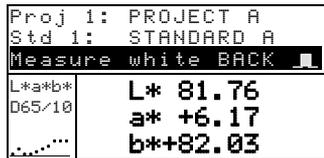
5. Measure the white backing of the opacity card. Release the instrument after the opacity value is displayed.
