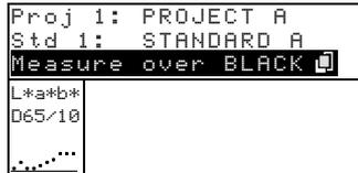
3. Measure the sample over the black portion of the opacity card. Release the instrument after data is displayed.
