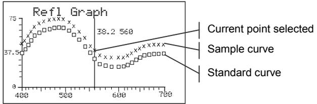
3. Repeatedly press the Tab Up key ↑ or Tab Down key ↓ to view the data in 10 nm increments, along the reflectance curve.
