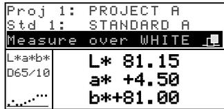
4. Measure the sample over the white portion of the opacity card. Release the instrument after data is displayed.
