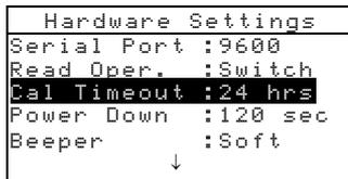
2. Press the Enter **↵** key to open the Set Cal Interval menu.
