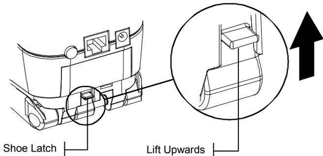
**To latch the Instrument Shoe:**
