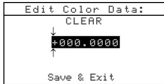
**NOTE:** Positioning the arrows above and below  $\uparrow$  or  $\downarrow$  and pressing the Enter key  $\leftarrow$  toggles between the two symbols.
