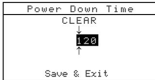
3. Use the Tab keys  $\updownarrow$  to choose the desired power down digit (arrows above and below designate selection). Press the Enter key  $\leftarrow$  to access the alphanumeric editor.
