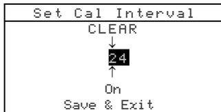
3. Use the Tab keys **↑↓** to choose the desired cal interval digit (arrows above and below designate selection). Press the Enter key **↵** to access the alphanumeric editor.
