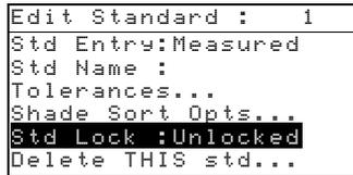
2. Press the Enter key ↵ to toggle between Locked and Unlocked. The “Delete THIS std” option only appears for an unlocked standard.
