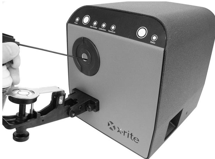
**IMPORTANT:** If can air is used for cleaning, do not invert or tilt the can during use. This could cause damage to the optics.
