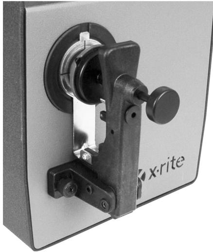
4. Initiate the white calibration procedure from the software application. The status indicator changes to amber. The calibration indicator should change to red.
