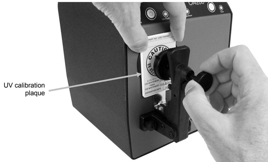
4. Close the sample holder clamp to the UV calibration plaque.
