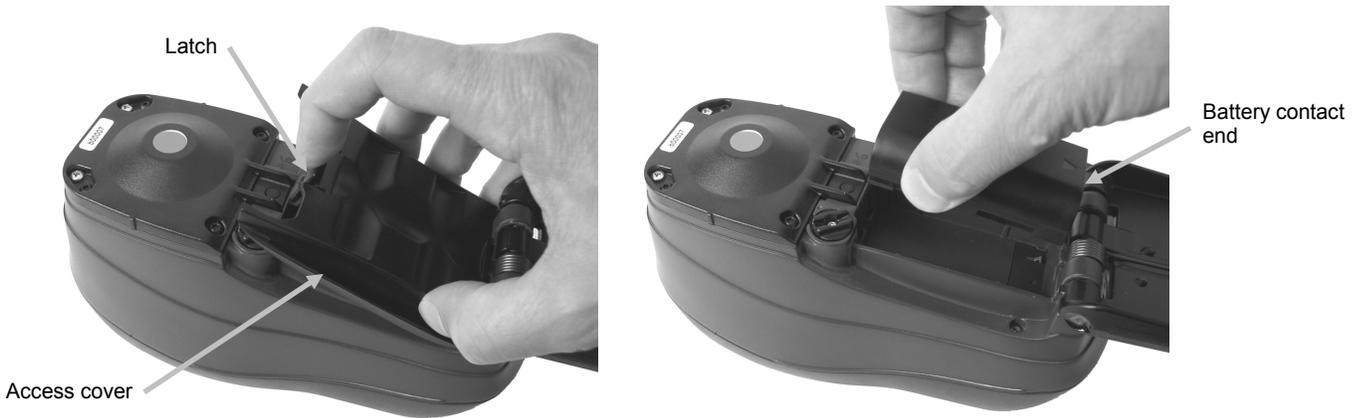
5. Reinstall the battery access cover by inserting the back edge first and then pressing downward until the access cover locks into position.
