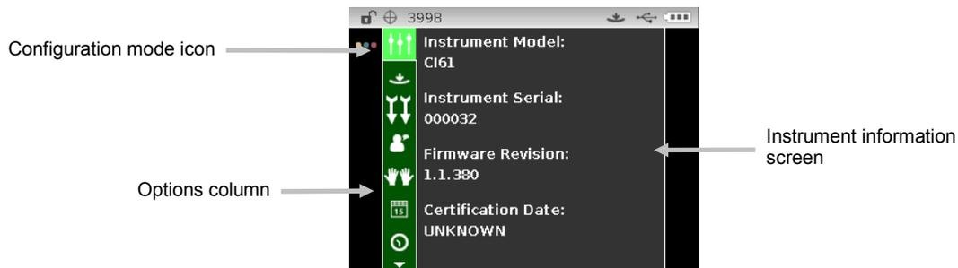
3. From the Configuration screen, use the **Up** or **Down** navigation buttons to move the highlight focus to the desired configuration icon in the Options column.
