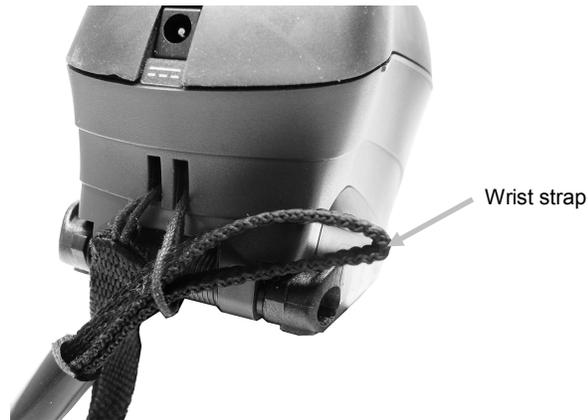
3. Pull on the wrist strap to secure to the strap post.
