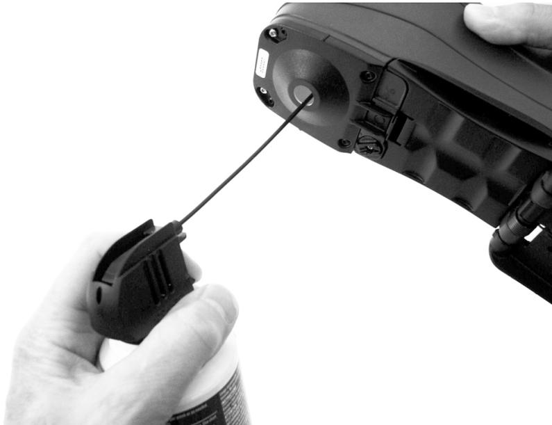
**IMPORTANT:** If can air is used for cleaning, do not invert or tilt the can during use. This could cause damage to the optics.
