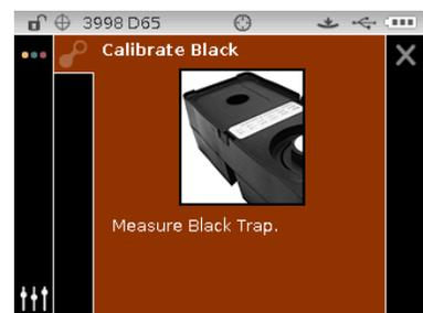
9. Press the instrument firmly to the shoe and hold steady until the display indicates that the reading is complete. Release the instrument.
