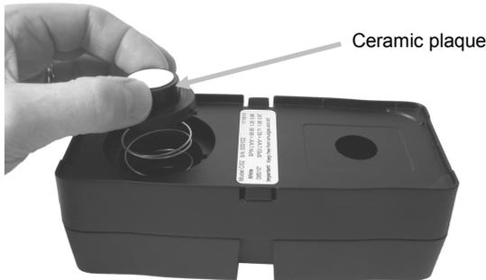
3. Clean the plaque using a mild soap and warm water solution. Thoroughly rinse with warm water and wipe dry with a lint-free cloth. Do not use solvents or cleaners of any kind.
