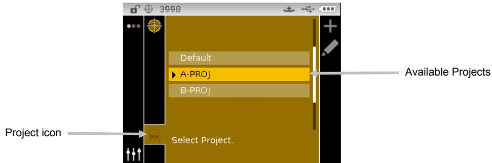
3. Use the **Up** or **Down** navigation buttons to move the highlight focus to the desired project.
