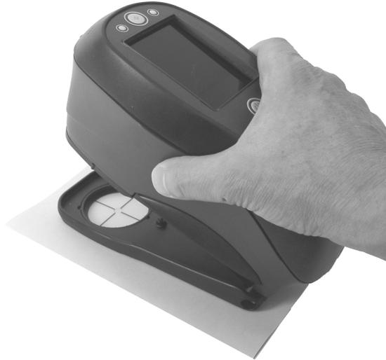
3. Press the instrument firmly to the shoe and hold steady until the display indicates that the measurement is complete.
