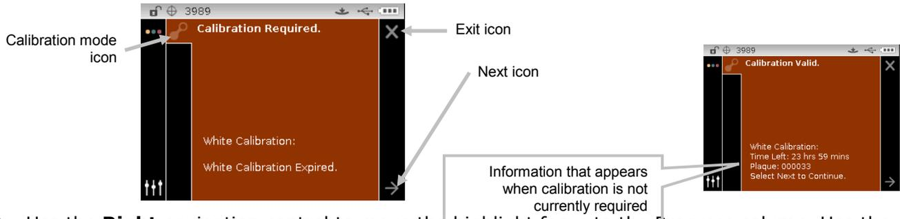
3. Use the **Right** navigation control to move the highlight focus to the Progress column. Use the **Down** navigation control to highlight the Next arrow icon (→) if not highlighted and tap the **Select** button.
