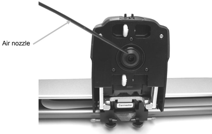
3. Lower the read head back to its measurement position and verify that the release posts snap back into position.
