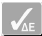
Best Match. Indicates if you can get a closer match to your color by adjusting the ink thickness for the color. When selected, the "best match" density value is displayed along with the Delta E for each color. The Delta E value is based on the calculated average for all zones.
