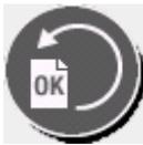
Touch to display the data for the OK sheet. The OK sheet is the target and all other sheets show target tolerances relative to the OK sheet data.
