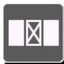
Manage Key. Allows you to shut off any unused or unwanted zones within the press for a specific ink unit. The bar graphs are then removed from the graphs for these zones and the data is
