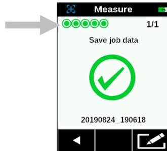
8. If the job was created on the instrument using the New Job feature, you can edit the name if desired. Tap on the Edit icon at the bottom of the screen and enter a job name using the virtual keyboard. Tap the Enter icon to save the job name.
