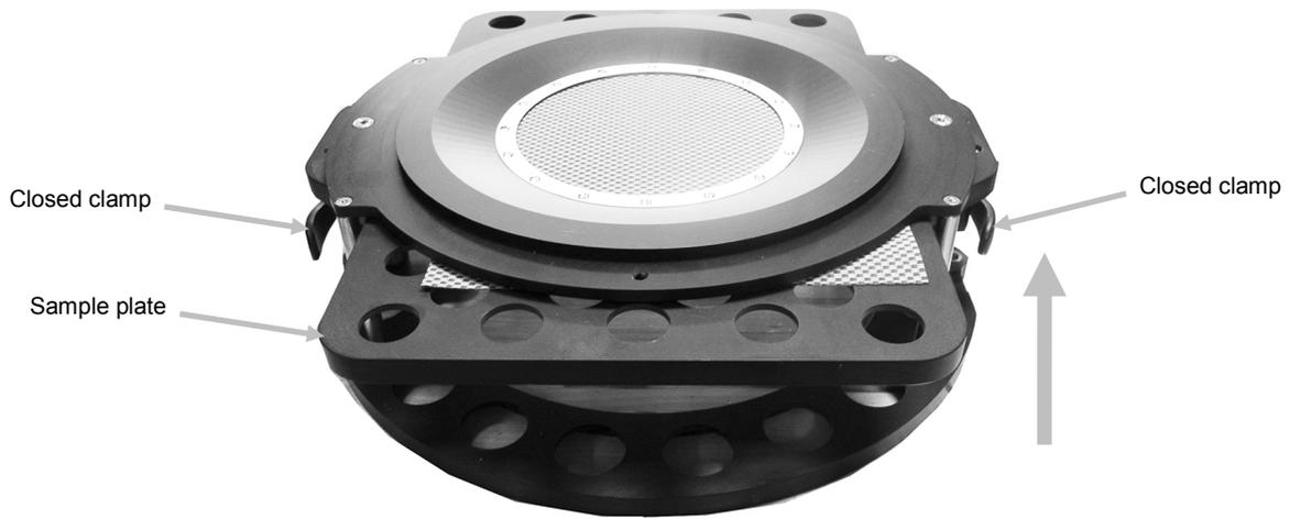
7. Insert cassette with sample into the drawer by placing the cassette over the alignment pins.
