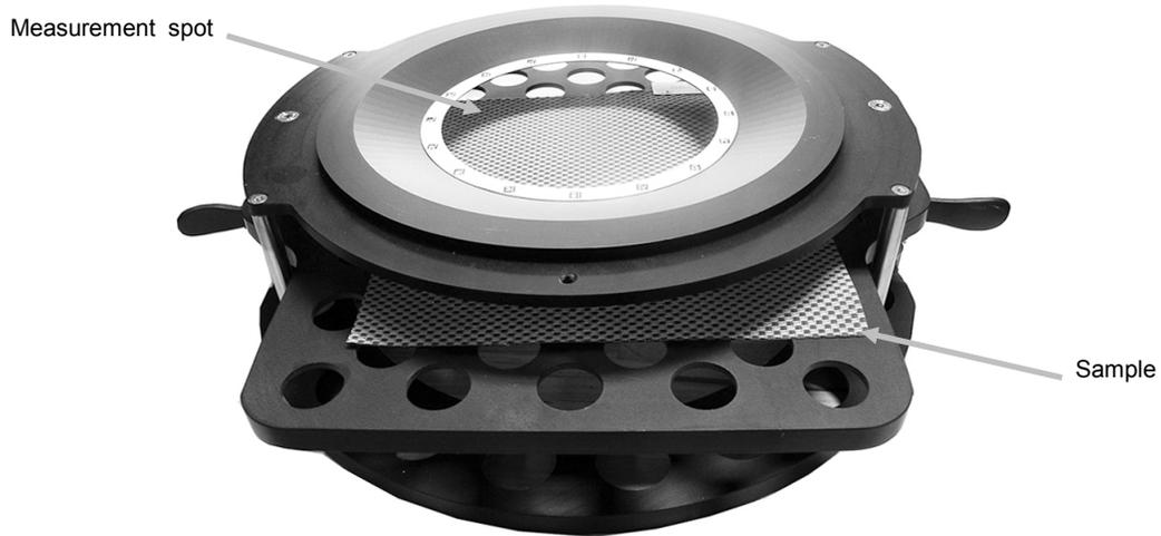
6. Lift the sample plate up until it stops against the measurement spot and close the cassette clamps.
