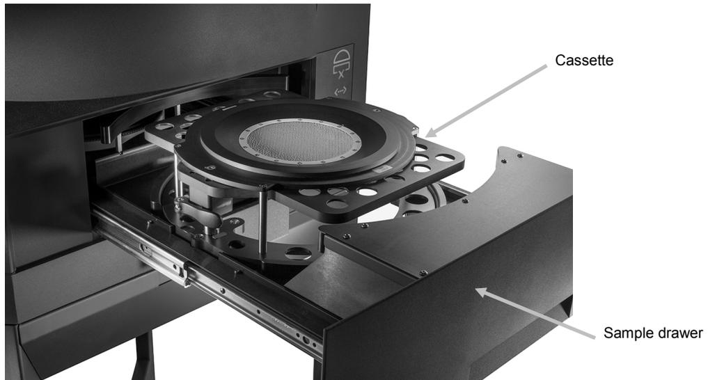
4. Place the cassette on a solid surface. If required open the clamps on the cassette and lower the sample plate.
