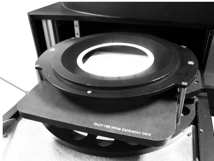
2. Lift the sample plate up until it stops against the measurement spot and close the cassette clamps.
