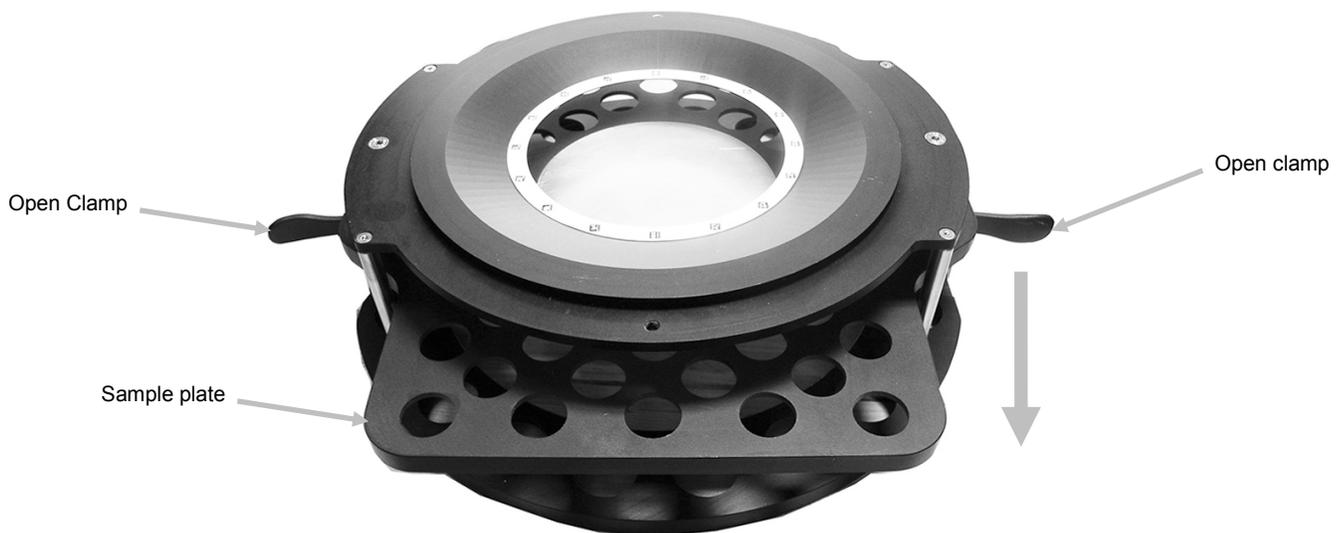
5. Place the sample on the sample plate in the cassette, and align the desired measurement area below the measurement spot.
