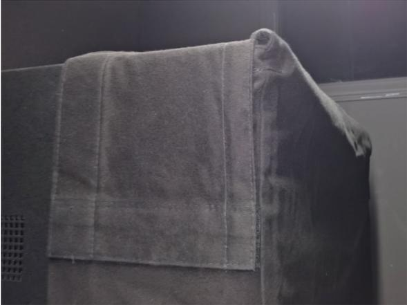
16. Hang the calibration curtain on the VLB so that the entire front is covered.
