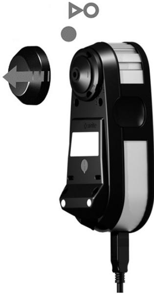
7. Open the protective slider on the calibration holder to access the white calibration tile.
