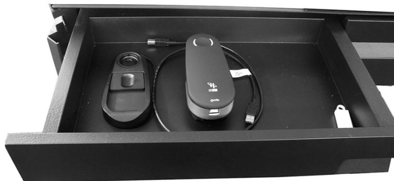
4. Plug the other end of the USB cable into the port on the front panel of the VLB.
