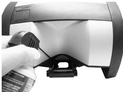
3. Position the instrument slider to the measurement position.
