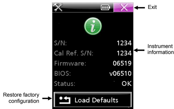
3. Press the right side of the **Navigation Ring** to quickly move the highlight focus to the **Exit** icon.
