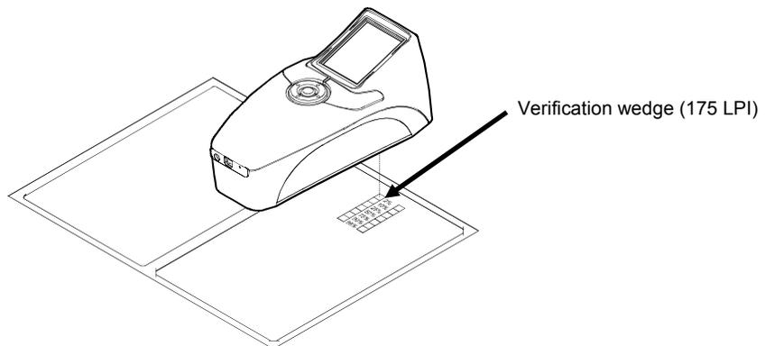
9. Press a **Measure** button to take the measurement. The screen displays a checkmark over the 2% patch if the patch was successfully measured.
