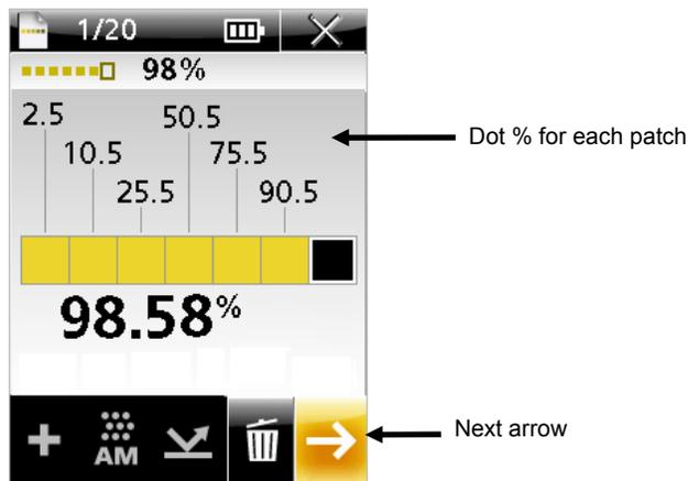
12. Use the **Navigation Ring** to move the highlight focus to **Next Arrow** icon and press the **Select** button. The screen returns to the main strip screen where the time and date stamp is displayed.
