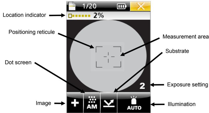
6. Locate the instrument’s target window on the **2% patch** of the target strip using the reticule icon in the screen for positioning.
