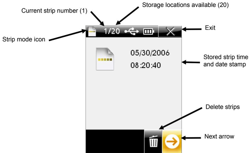
3. Activate targeting mode by pressing the **Measure** button; or use the **Navigation Ring** to move the highlight focus to the **Next Arrow** icon and press the **Select** button.
