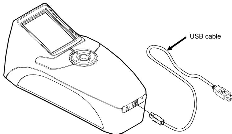
**IMPORTANT:** Never unplug the USB cable when data is being transferred to the computer.
