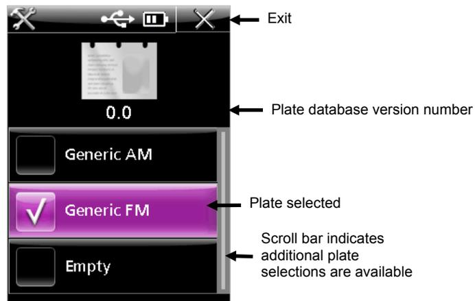
3. Use the **Navigation Ring** to move the highlight focus to the desired plate icon. Additional plates not displayed are accessed by continually pressing on the bottom or top of the Navigation Ring.
