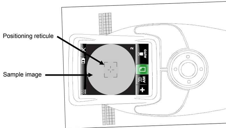
The instrument must be positioned flat on the sample and remain still through the entire measurement.
