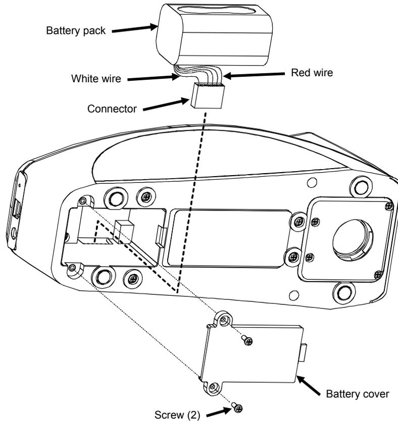
5. Remove the old battery pack and unplug the connector.
