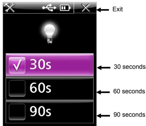
3. Use the up and down sides of the **Navigation Ring** to move the highlight focus to **30s**, **60s**, or **90s** icon.
