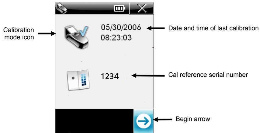
3. Activate targeting mode by pressing the **Measure** button; or press the **Select** button while the **Begin Arrow** icon is highlighted.
