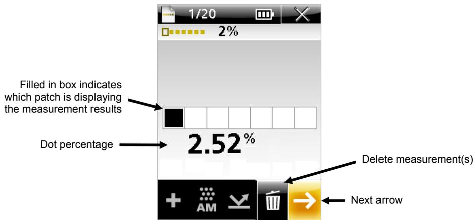
If a mistake was made and you would like to re-measure the patch, use the **Navigation Ring** to move the highlight focus to **Delete** icon and press the **Select** button. The last measurement taken on the strip will be deleted. Each patch is deleted individually, starting with the last measured.
