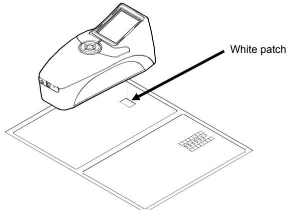
5. Press a **Measure** button to take the measurement. The screen displays a “checkmark” over the patch icon if the patch was successfully measured.
