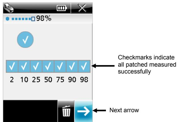
**NOTE:** A minus symbol (-) may appear in the patch location if the measurement failed or the patch was skipped.
