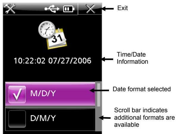
3. Use the **Navigation Ring** to move the highlight focus to the desired format.
